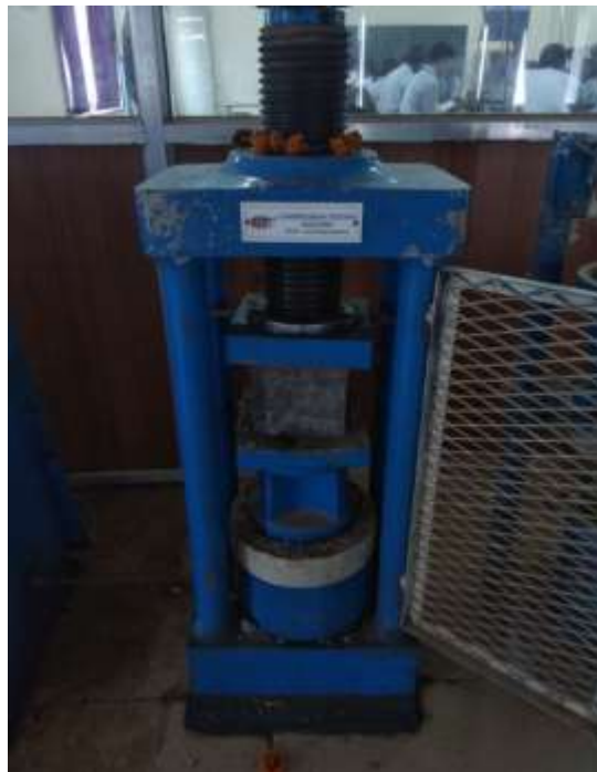
Fig 2. : Compression test on Cube
