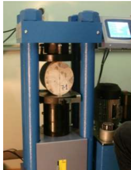
Fig 6 : Split tensile test on cylinder
