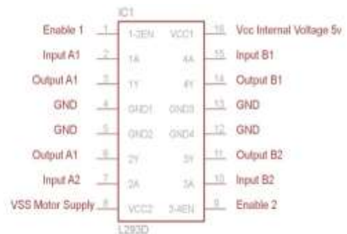
Fig-7: Motor drive (L293D)
