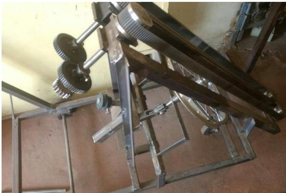
Fig No 1: Experimental setup of groundnut pod separating and removing machine
