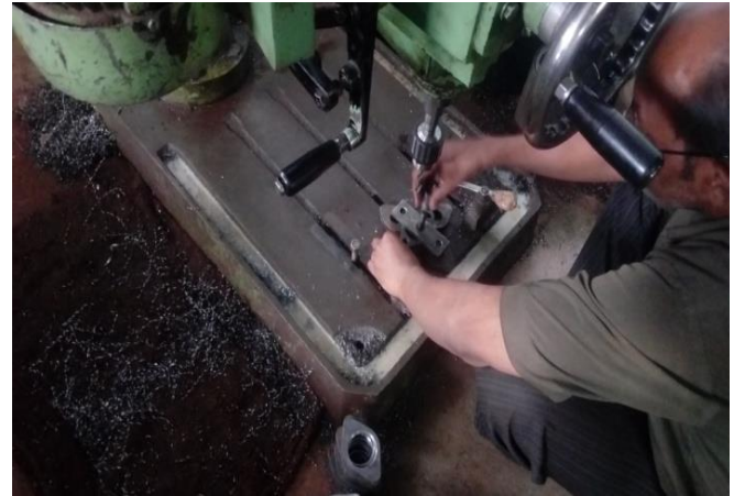
Fig.3 Job adjustment on drilling machine
