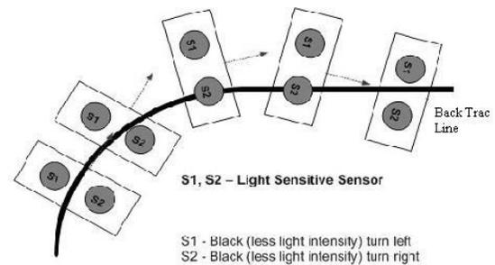
Fig 3: Module of Line Sensing
