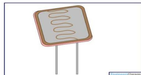
Fig 5:-Pin Diagram LDR
