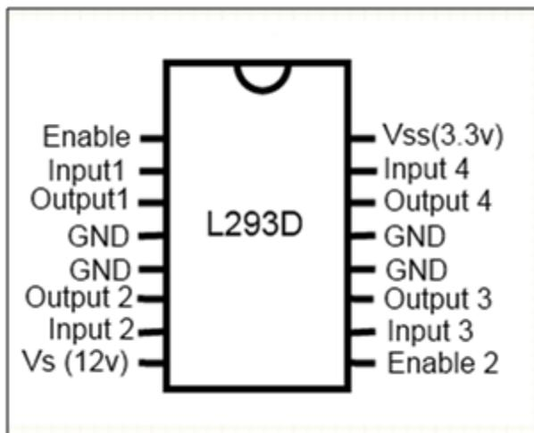
Fig 6:-Pin Diagram L293d
