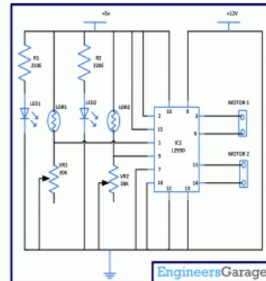
Fig 9: Circuit diagram by using L293d
