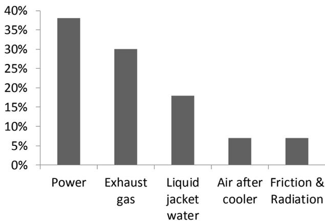
**Fig.1 Amount of heat dissipated from the engine [3]**
