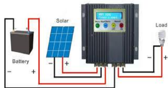
Fig-4: Charge Controller
