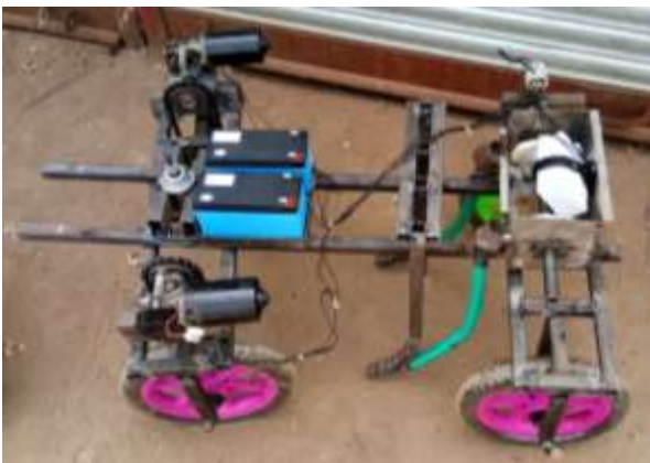
Fig-1: Actual Model of Remote Operated Seed Sowing Machine
