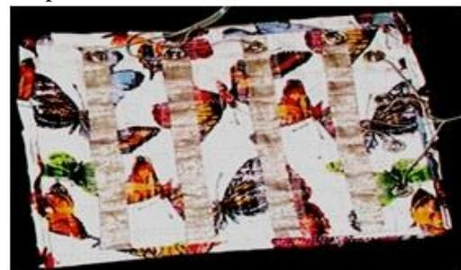
Fig-3.2(a): Fabric switching contact keyboard
