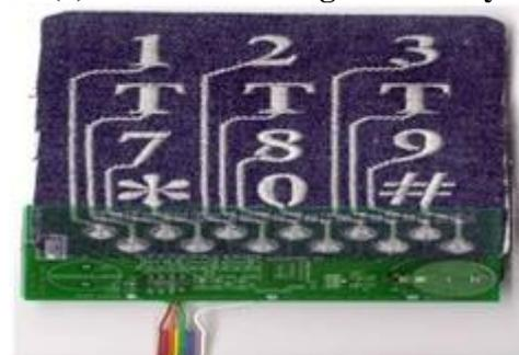
Fig-3.2(b): Capacitive keyboard
