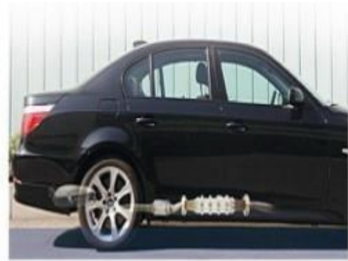
Fig-7.2: Renault prototype vehicle using TEG waste heat recovery
