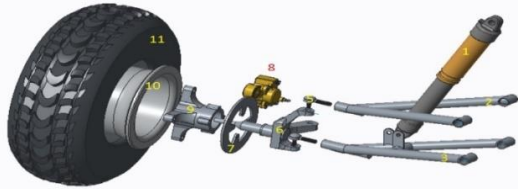
Fig-1: Exploded View of Double Wishbone Suspension System
