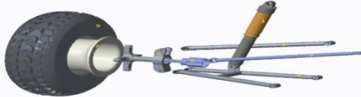
Fig-2: Exploded View of rear suspension system
