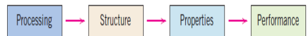
The four components of the discipline of materials science and engineering and their interrelationship.
