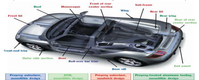
Fig-4: CFRP (Carbon fibre reinforced polymer) Application [1]
