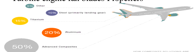
Fig- 07: The Boeing 787 Dreamliner Is 50% Composite Materials
