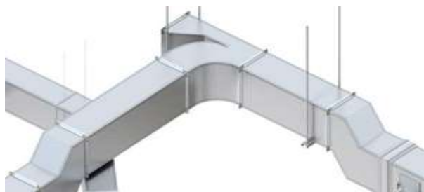
Figure 1.1: Rectangular Duct with sudden contraction and turns.
