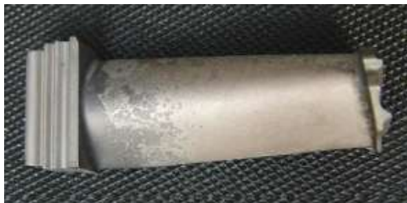
Fig. 3.3 Sulphidation attack of a turbine blade. Such damage can sometimes be repaired by removing the damaged coating and reapplying new coating.
