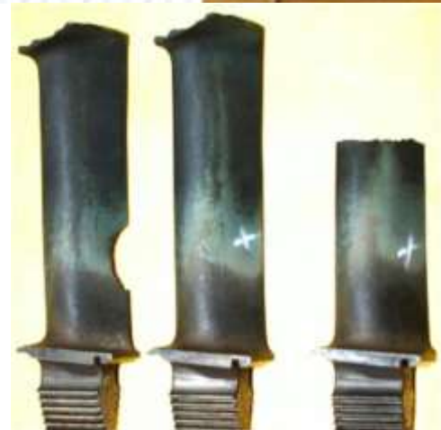
Fig. 3.4 Thermal failure of gas turbine blade
