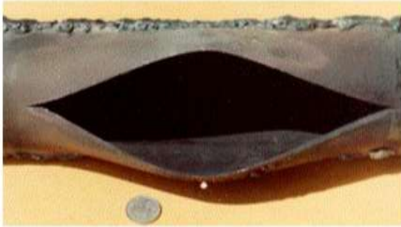
Fig. 1. Import Steam Super Heater Tubes of Boiler SGP NFL Naya Nangal.
