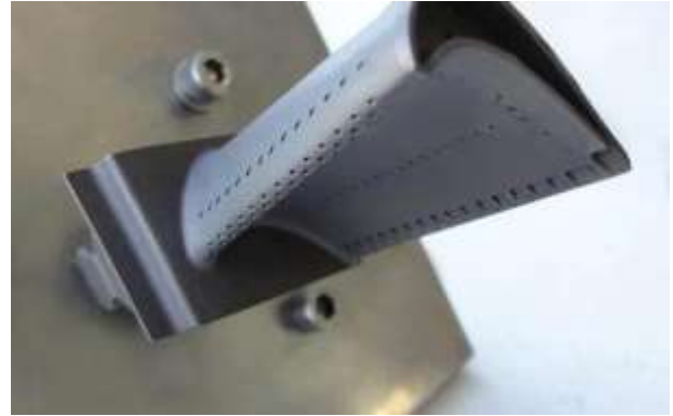
Fig: 4.3. Turbine blade with cooling passage
