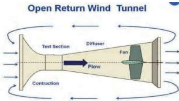
Fig. 2. Diagram of an open circuit, also known as wind tunnel.
