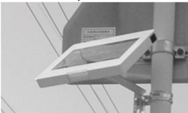
Fig-5: Bluetooth tags with solar battery on traffic signpost
