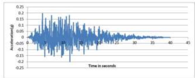
**Fig. 6: IS code ground motion with PGA scaled to 0.2g and duration equal to 40 seconds**
