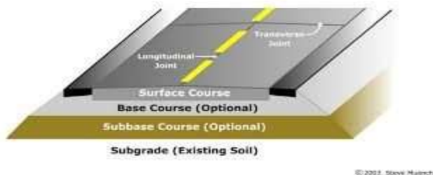
Fig.3: component of flexible pavement
