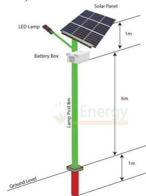
Fig. Solar Street Light Dimensions and Labels
