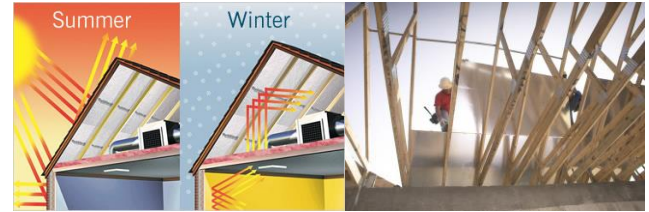
Fig 4: Radiant Barrier Sheathing
