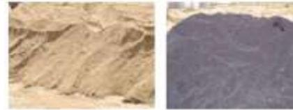
**Fig 1: Fine Aggregate and Copper Slag**
