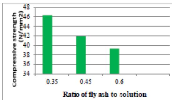
Fig.2 Effect of varying alkaline liquid to fly ash ratio on 7 days compressive strength
