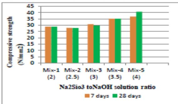
Fig.3 Effect of sodium silicate to sodium hydroxide ratio on compressive strength on GPC
