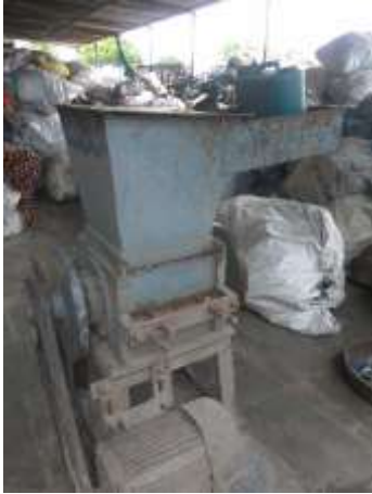
Fig-8: Plastic waste cutting machine.
