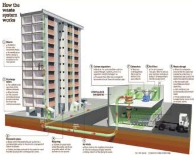
Fig-5: pneumatic waste collection.
