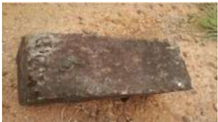
Fig 7: - Papercrete brick after fire test
