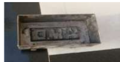
Fig4: - Mould used for casting of the brick
