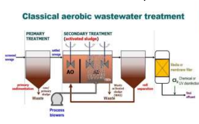
Fig-1 Aerobic wastewater treatment
