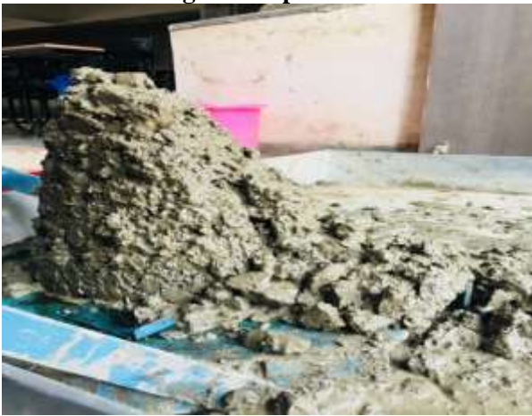
Fig-2 Slump Control mix
