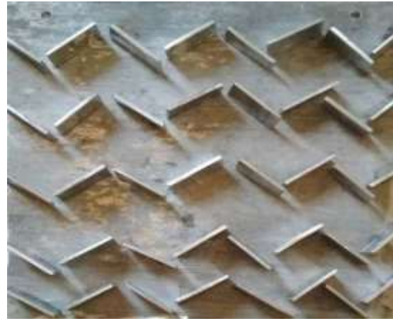
Fig.4 Vertical plate with short length V-type fins .
