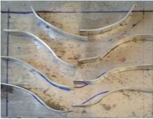
Fig. 3 Vertical plate with S fins
