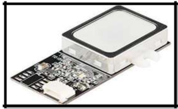
Fig.5.2 Finger Print Sensor
