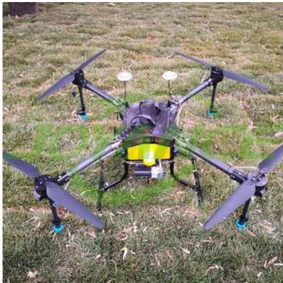
Fig-5: Complete View of assemble drone mounted sprayer
