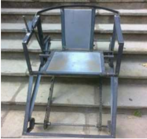
Fig4. working model of stair climbing wheel-chair[4]
