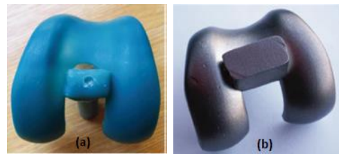
Fig.1 (a) prototype of Wax Pattern for investment Casting (b) Prototype of a new metal knee joint replacement [11].
